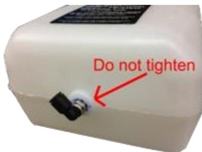
**Note:** All tanks are tested for leaks during assembly. A special sealant adhesive is used to bond the plastic tank to the metal fitting. **DO NOT** attempt to tighten the fitting any further!
