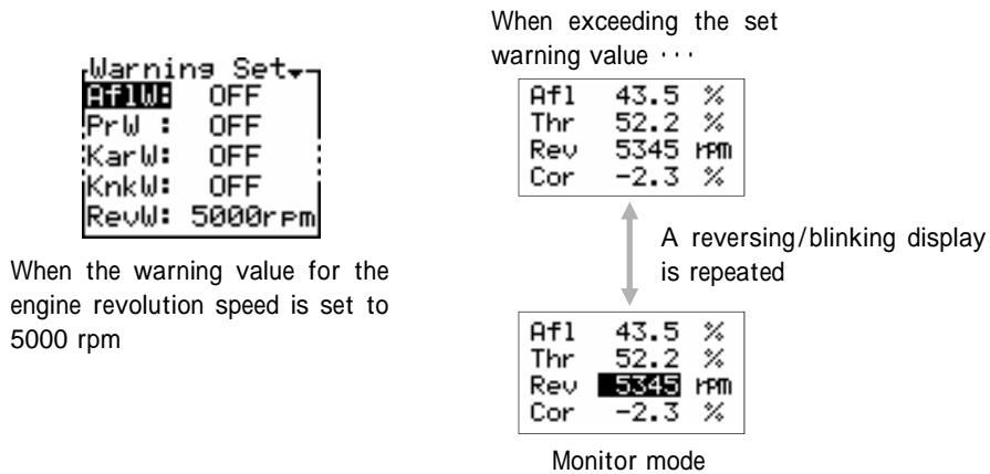
When the warning value for the engine revolution speed is set to 5000 rpm
