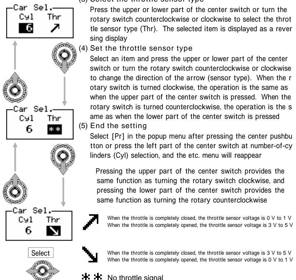
Set the throttle sensor type after checking the voltage in the completely closed/opened status of the throttle in the sensor voltage check mode described on the next page
