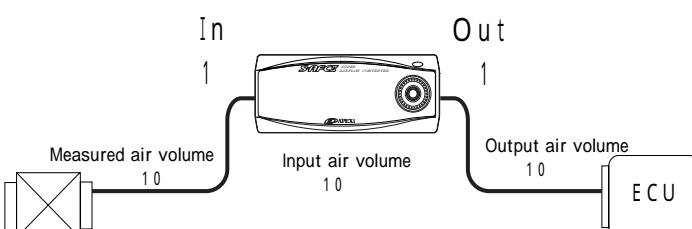
In this case, the airflow sensor measures an air volume of 10
