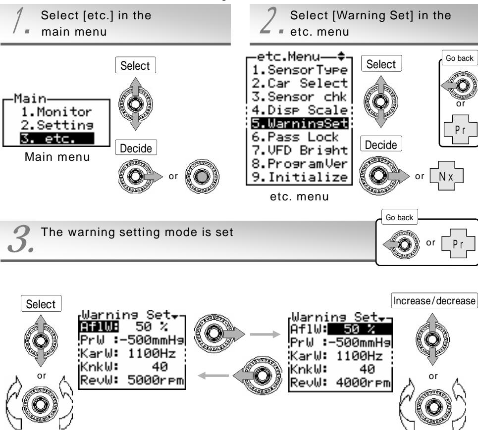
When the unit of pressure display is set to pascal (kPa) in the display scale setting on the previous page, the unit of pressure warning in this item is changed into pascal (kPa)
