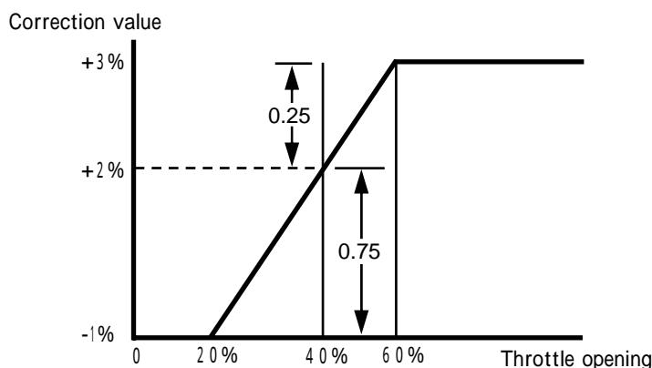
The air correction factor at a throttle opening of 40% can be obtained by the following formula
