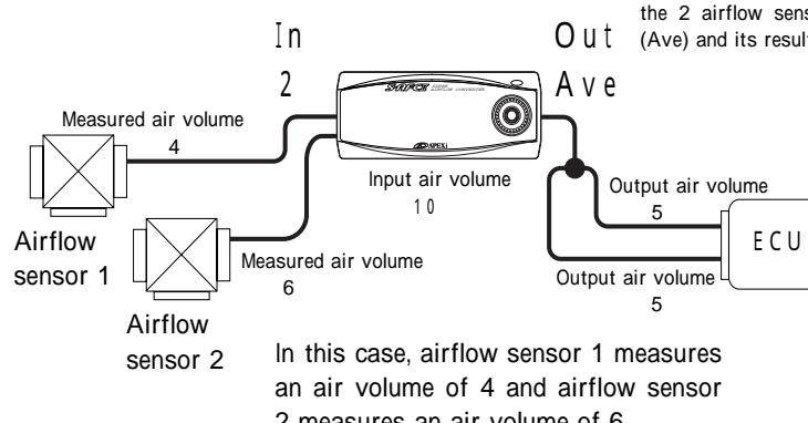
Because of 2 engine control unit inputs, the measured air volume of the 2 airflow sensors is averaged (Ave) and its result is output
