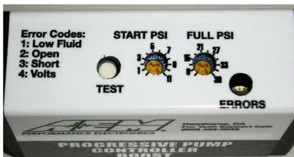
Adjust the “Start PSI” value by setting the dial to approx 25% of the vehicles maximum boost. Adjust the full-in value to your maximum boost (up to 38 PSI of boost).
